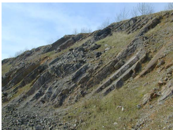
Fig. 6.23 Interesting low angle final face produced by stepped blasting
