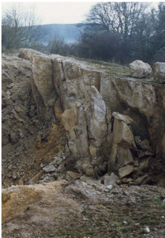
Fig. 5.8 Toppling of blocks in a limestone quarry
