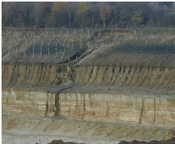
Fig. 5.11 Rotational failure through saturated superficials overlying clays and sand deposits
