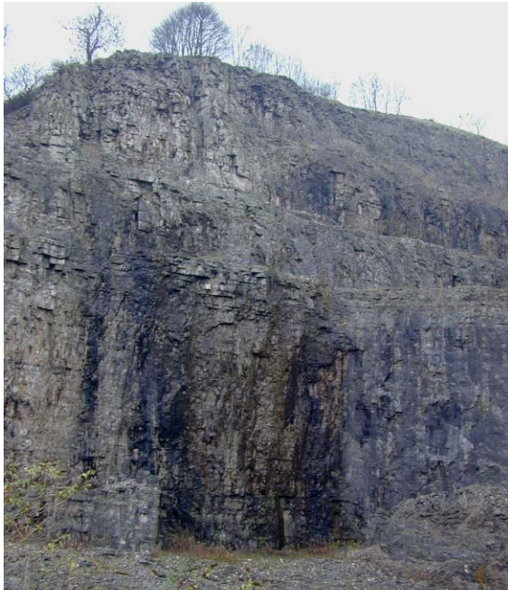
Fig. 6.49 High bench faces with no on-bench access and active rockfall
