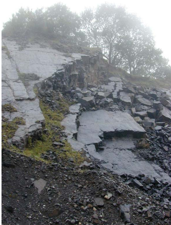
Fig. 5.4 Planar instability in a limestone quarry resulting from undercutting of bedding by excavation
